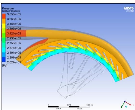
Figure 13 - Optimised Design Static Pressure Contour at Diffuser Mid Height.
