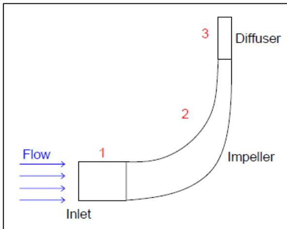
Figure 8 - Impeller Computational Domain
