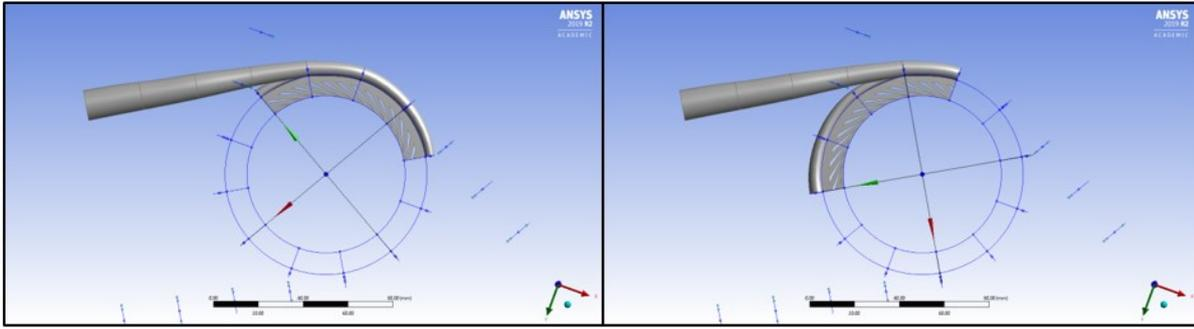
Figure 10 - Domain Slice at 0 and 60 Degrees Forward of Tongue
