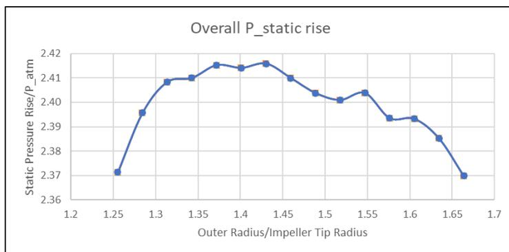
Figure 9 - Static Pressure Rise With Diffuser Radius: Vaneless Diffuser
