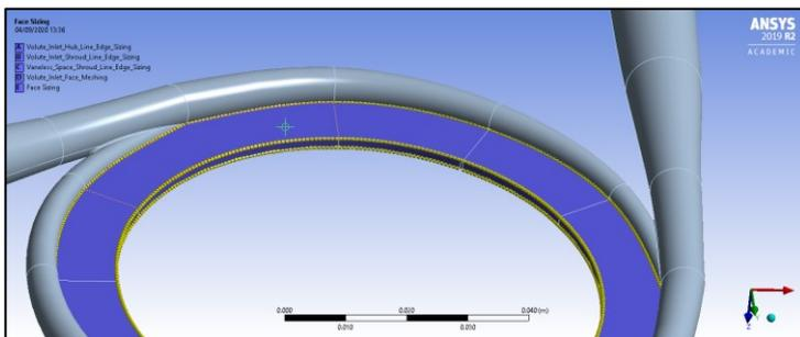
Figure 7 - Volute Mesh Line Sizing
