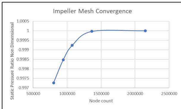
Figure 6 - Impeller Mesh Convergence
