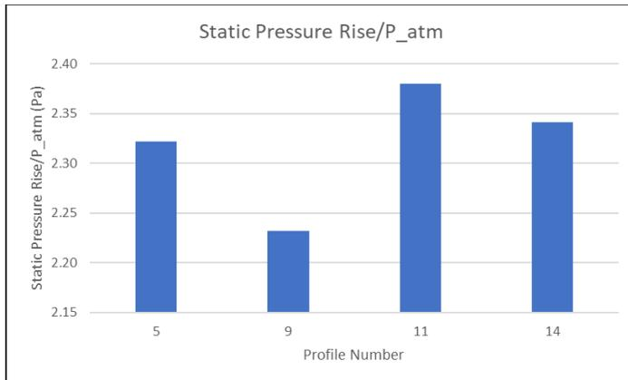
Figure 4: Static Pressure Rise in Different Volute Shapes
