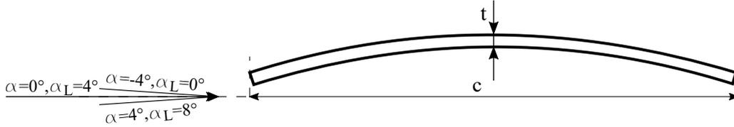
Figure 5: Cambered plate with relative camber  $h/c = 8\%$ , with indication of the maximum blade thickness  $t$  and the chord length  $c$ . The angle of attack  $\alpha$ , and the zero lift based angle of attack  $\alpha_L$  is represented with three examples
