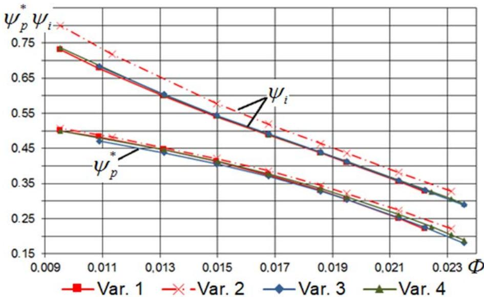
**Figure 5: Polytropic work coefficient and work coefficient of the stage with vaneless diffuser candidates 1- 4**
