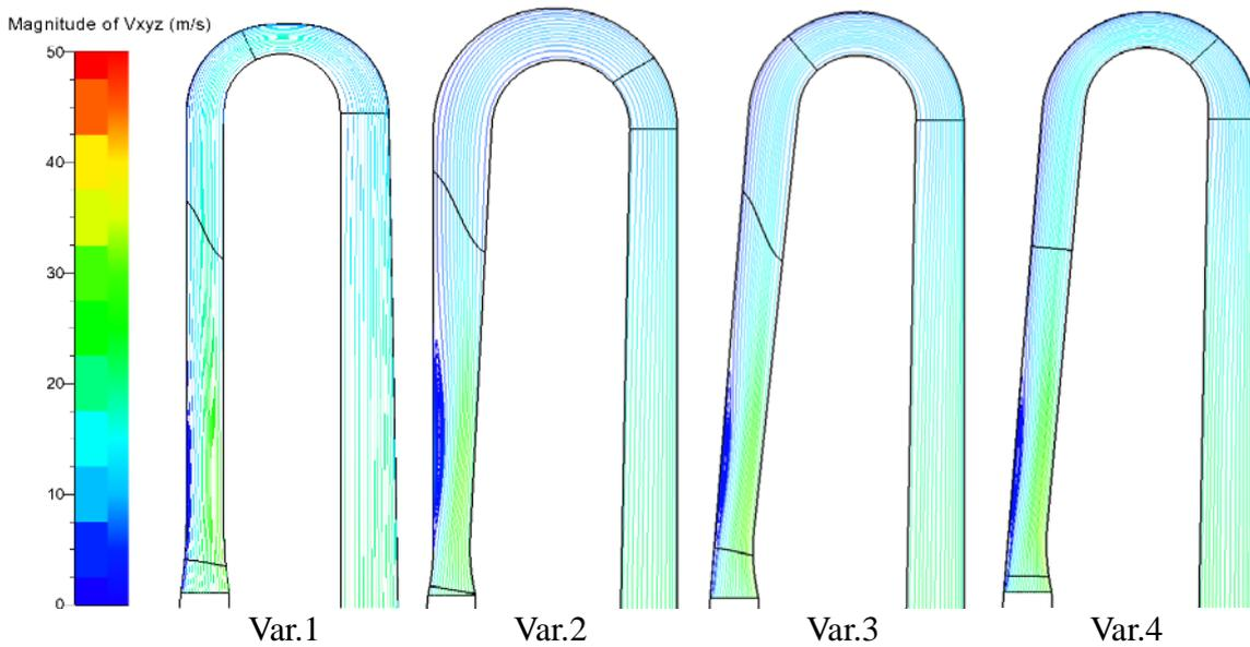
**Figure 6: Stream lines in vaneless diffusers and return channel at the design flow rate**
