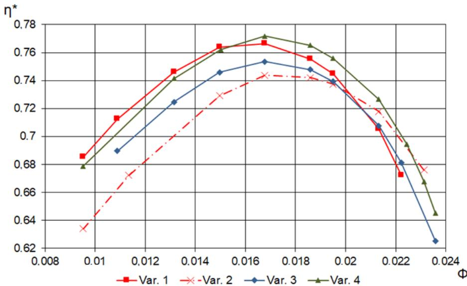
**Figure 4: Efficiency of the stage with vaneless diffuser candidates 1- 4**
