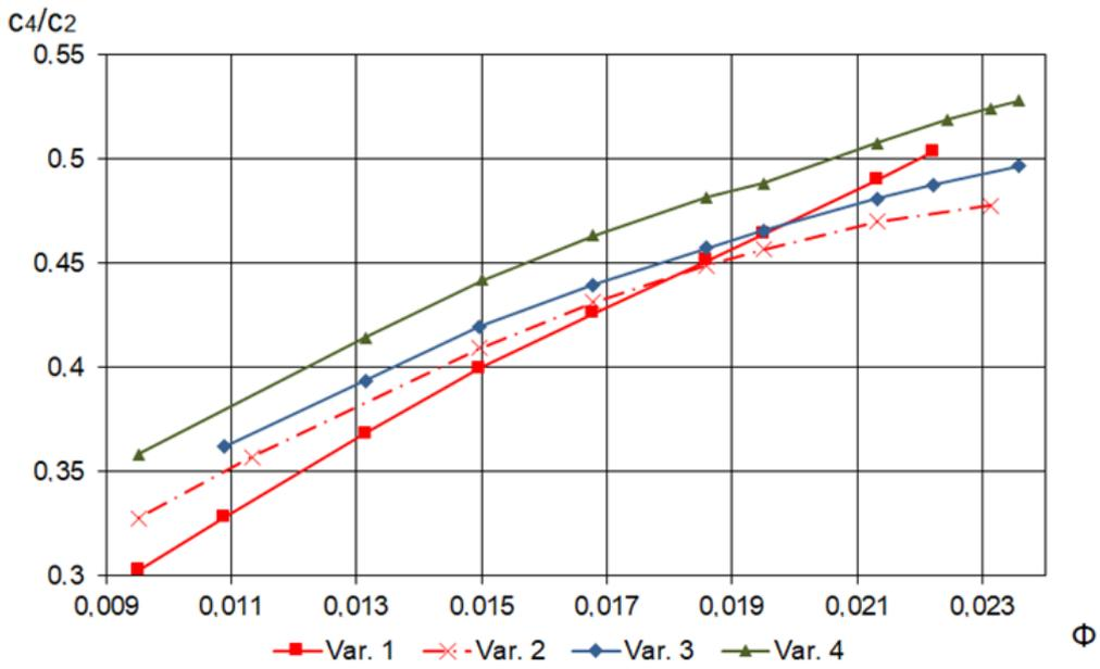
Figure 9: Velocity ratio in vaneless diffusers 1 - 4
