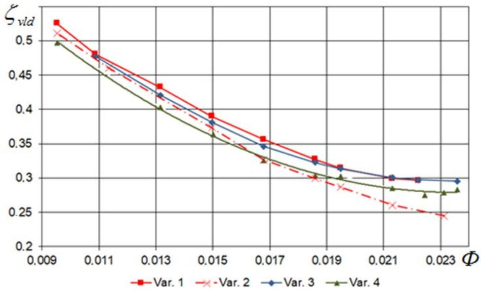
Figure 8: Loss coefficients of vaneless diffusers 1 – 4
