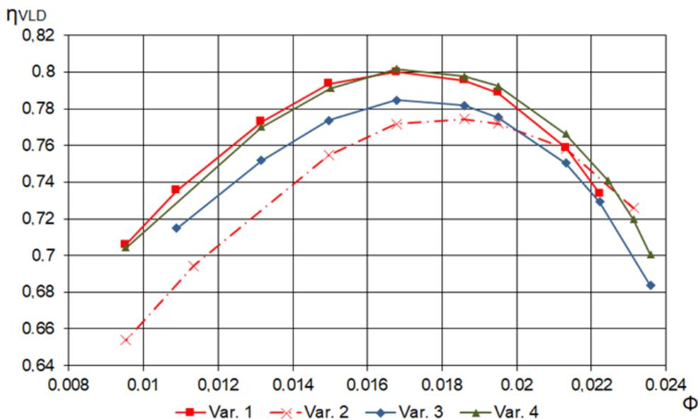
**Figure 7: Efficiency of vaneless diffusers 1 - 4**
