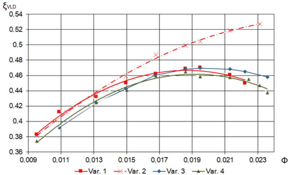
**Figure 10: Recovery coefficients of vaneless diffusers 1 – 4**
