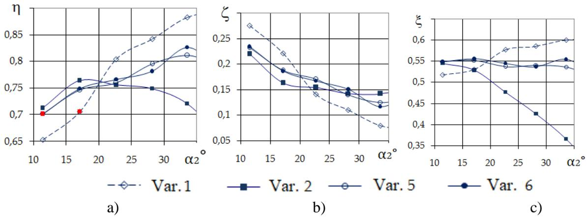
**Figure 2: VLD candidates' characteristics a) efficiency, b) loss coefficient, c) recovery coefficient**
