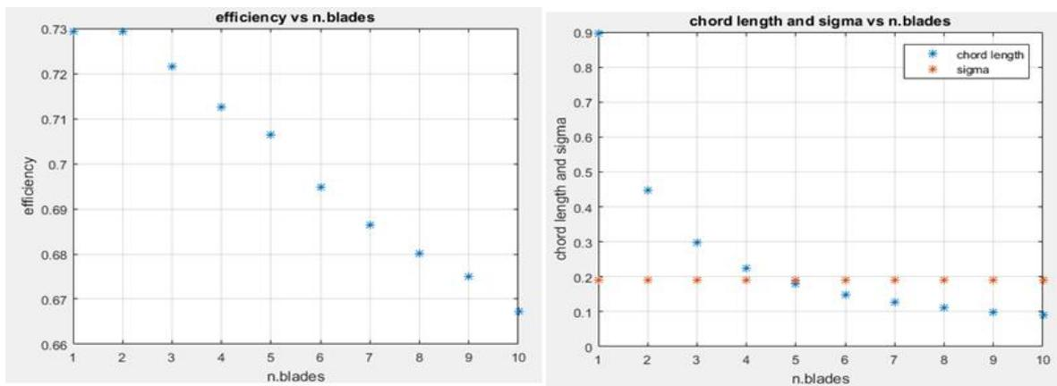
**Figure 5 : 1D optimal solution for different number of blades. Efficiency (left figure), Chord length and Solidity (right figure) as a function of the number of blades**
