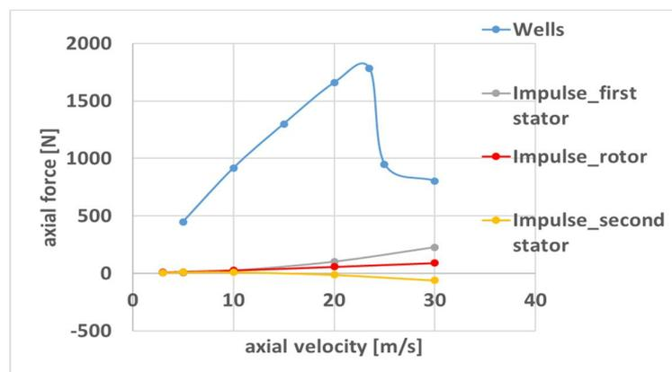
**Figure 14 : per blade axial loads for Wells and Impulse turbine**
