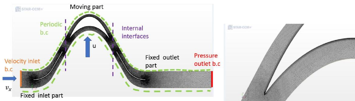
**Figure 9 : geometry and mesh for the impulse turbine CFD simulations**
