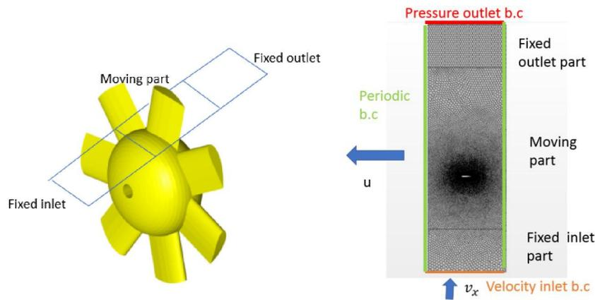
**Figure 3: geometric domain for CFD simulation and the mesh used with its boundary conditions**
