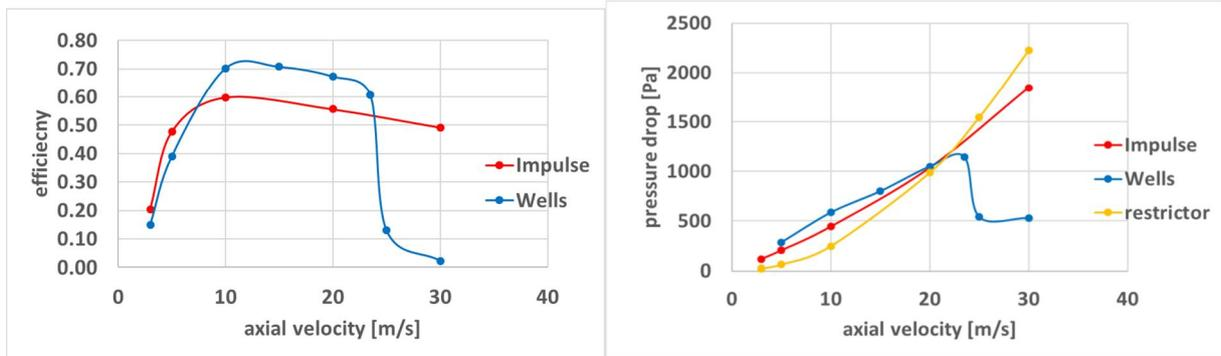
**Figure 13 : efficiency and pressure drop of Wells and Impulse turbine as a function of axial velocity**
