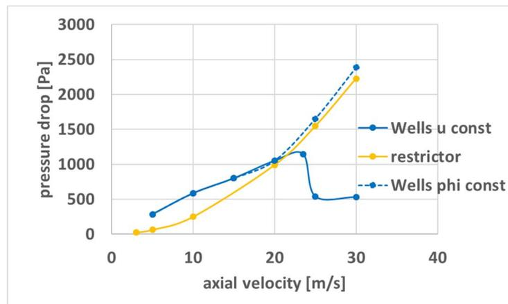
**Figure 6: pressure drop as a function of axial velocity for Wells turbine compared to the restrictor**
