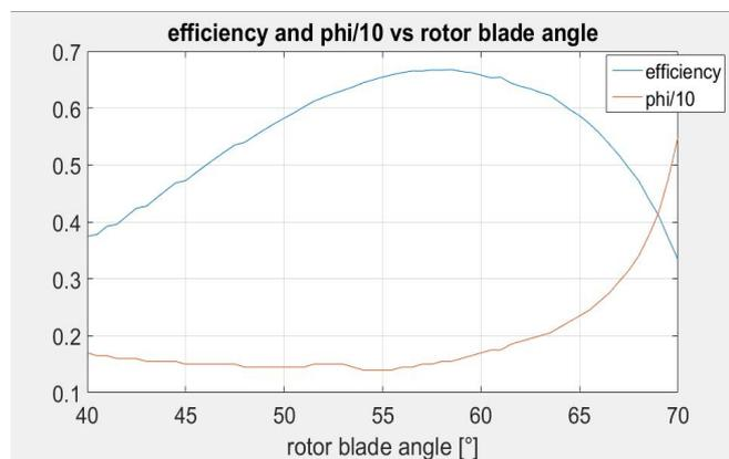
**Figure 8 : efficiency and flow coefficient/10 as a function of rotor blade angle (measured from the axial direction)**
