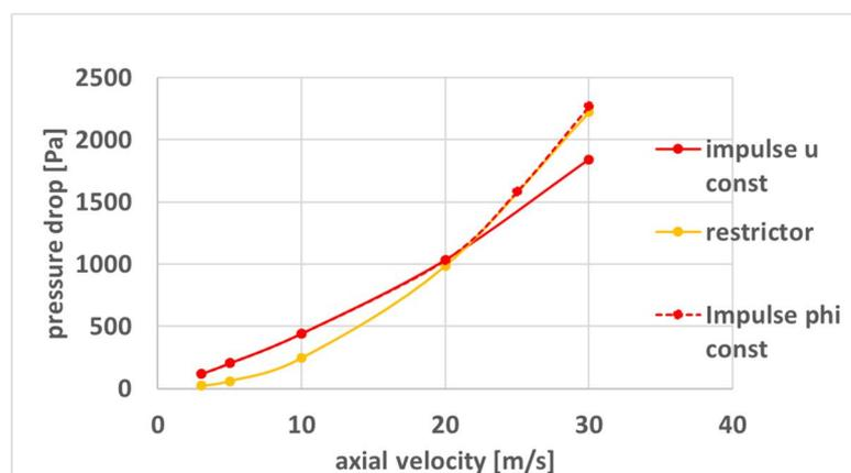
**Figure 12 : pressure drop of impulse turbine compared to the restrictor**
