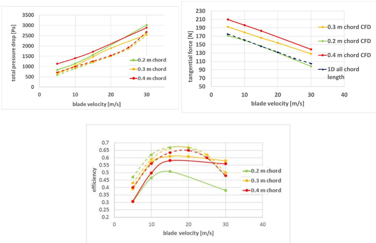
**Figure 10 : total pressure drop, tangential force , efficiency for a 40 blades impulse turbine according to 1D Code (dashed lines) and CFD (continuous lines)**
