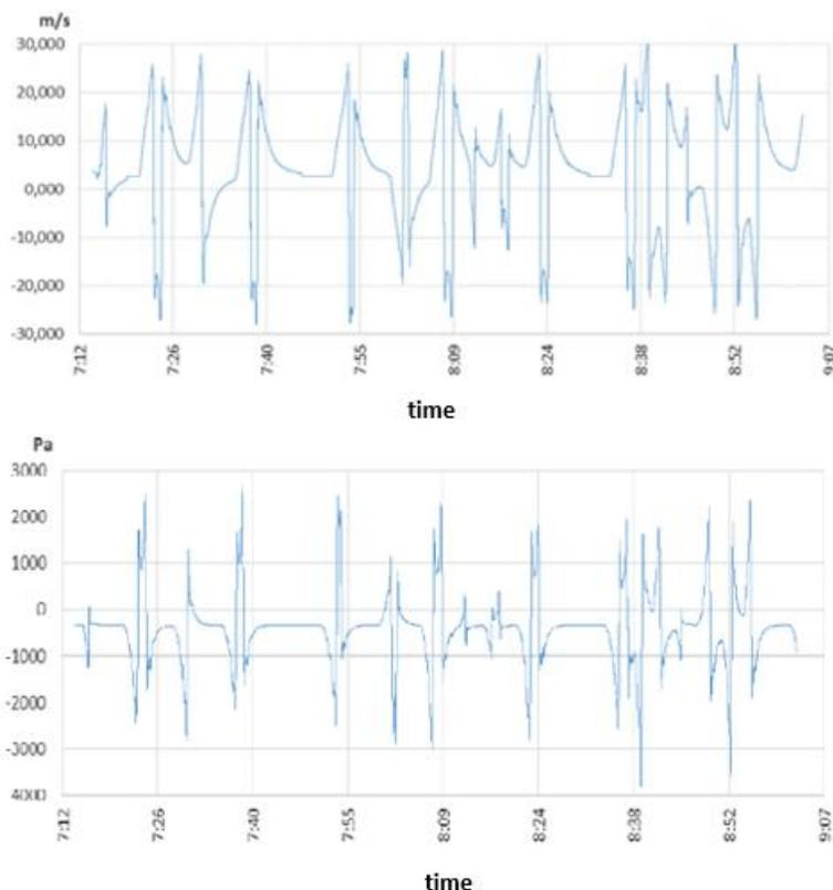
**Figure 1: Instantaneous velocity and pressure drop measured in the PRD (Division Infrastructure Eurotunnel 2010)**
