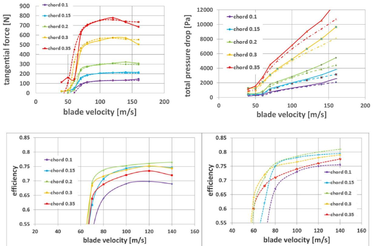
**Figure 4: tangential force, total pressure drop and efficiency of the 8 blades Wells turbine according to 1D (dashed curves) and CFD models (continuous curves)**
