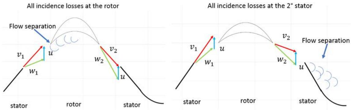
**Figure 7: two extreme angles configurations for impulse turbine**
