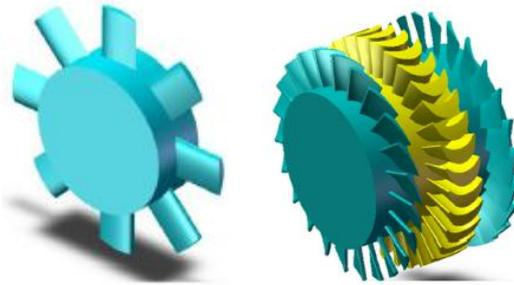
**Figure 2: self-rectifying turbines: on the left Wells turbine, on the right Impulse turbine from[[www.scoop.it/turbines/p/4007344956/2013/09/09/numerical-analysis-of-impulse-turbine-for-isolated-pilot-owc-system](http://www.scoop.it/turbines/p/4007344956/2013/09/09/numerical-analysis-of-impulse-turbine-for-isolated-pilot-owc-system)]**
