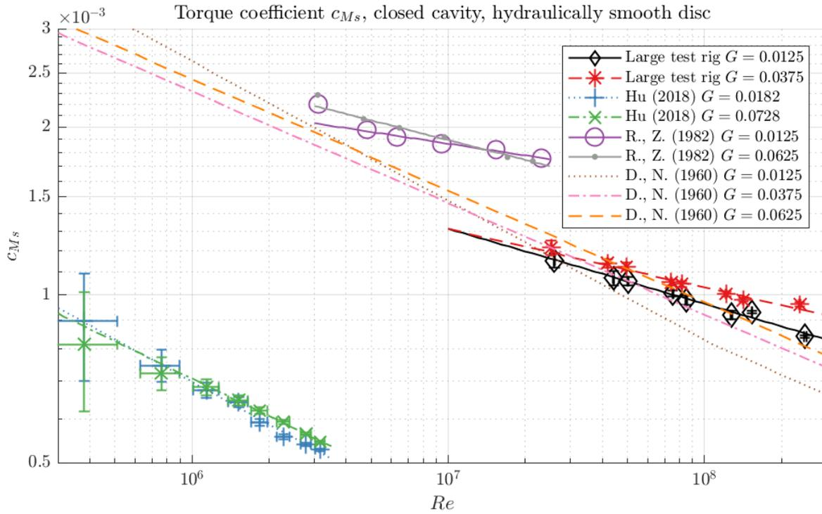
**Figure 2: Torque coefficient of a closed rotor-stator cavity with hydraulically smooth disc. Lines belonging to measurement points are curve fits. “R., Z. (1982)” refers to Radtke and Ziemann (1982), “D., N. (1960)” refers to Daily and Nece (1960).**
