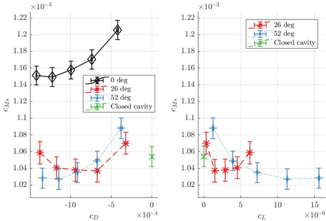
**Figure 8: Torque coefficient  $c_{Ms}$  for relative gap width  $G = 0.0375$  and Reynolds number  $7.5 \cdot 10^7 \leq Re \leq 9.6 \cdot 10^7$  of closed cavity as well as three different preswirl angles.**
