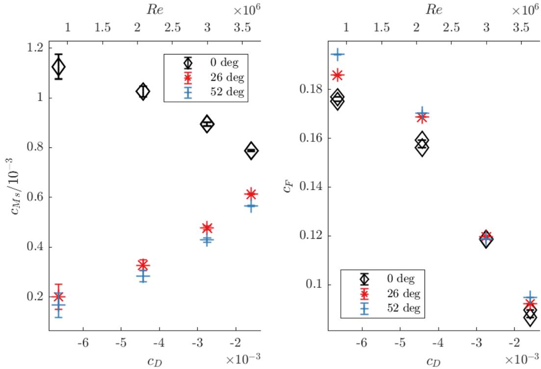
**Figure 11: Influence of preswirl angle on torque and moment coefficient in the small test rig (compare Hu (2018)) with relative cavity width  $G = 0.0182$ . For the results shown here, the product  $c_D \cdot Re$  is constant.**
