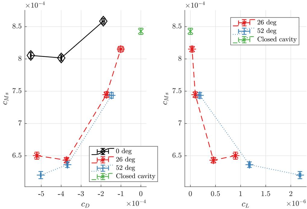
**Figure 6: Torque coefficient  $c_{Ms}$  for relative gap width  $G = 0.0125$  and Reynolds number  $1.8 \cdot 10^8 \leq Re \leq 2.9 \cdot 10^8$  of closed cavity as well as three different preswirl angles.**
