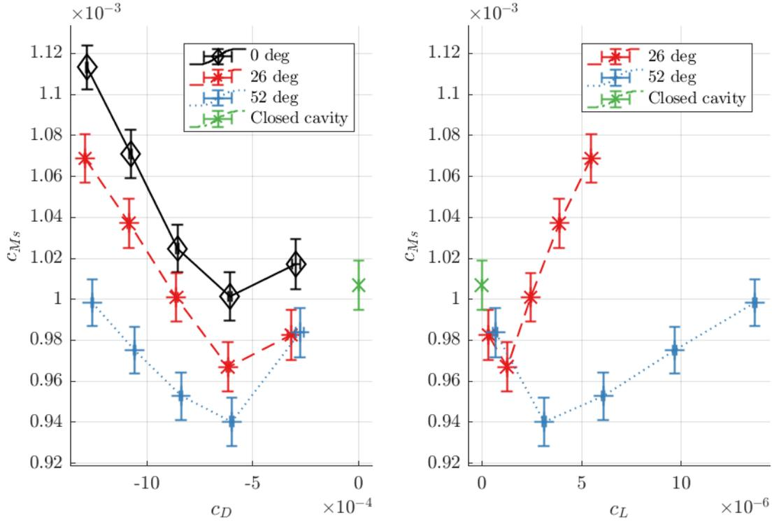
**Figure 5: Torque coefficient  $c_{Ms}$  for relative gap width  $G = 0.0125$  and Reynolds number  $7.5 \cdot 10^7 \leq Re \leq 9.6 \cdot 10^7$  of closed cavity as well as three different preswirl angles.**
