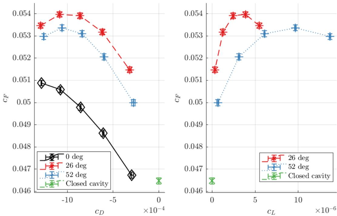
**Figure 7: Axial thrust coefficient  $c_F$  for relative gap width  $G = 0.0125$  and Reynolds number  $7.5 \cdot 10^7 \leq Re \leq 9.6 \cdot 10^7$  of closed cavity as well as three different preswirl angles.**
