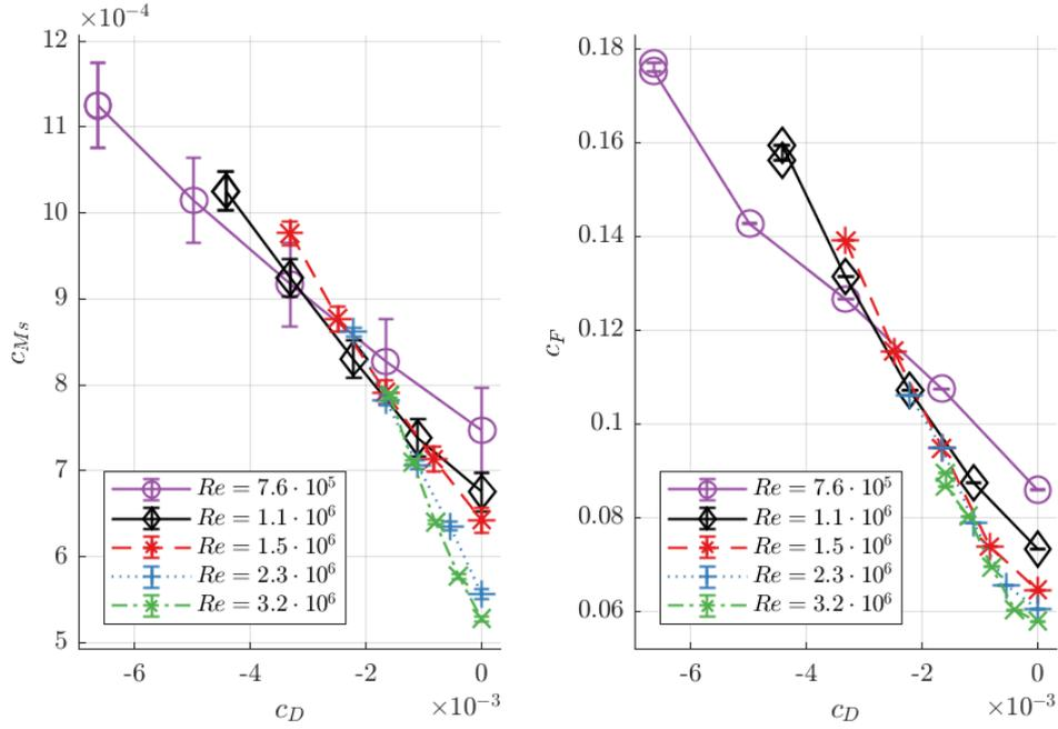
**Figure 10: Axial thrust coefficient  $c_F$  and torque coefficient  $c_{M_s}$  measured in the small test rig (compare Hu (2018)) with closed cavity ( $c_D = 0$ ) and radial inflow ( $\alpha = 0$ ,  $c_D < 0$ ) for the small relative cavity width  $G = 0.0182$ .**
