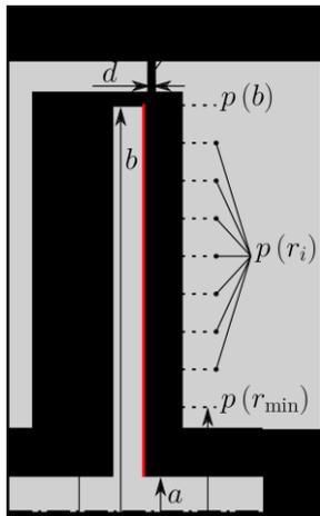
**Figure 1: Schematic of the Rotor-stator cavity test rigs used. Dashed lines indicate pressure measurements, torque coefficients  $c_{Ms}$  correspond to the torque acting on the surface indicated by the red line. The small test rig does not have a hub in its front cavity according to Hu (2018).**
