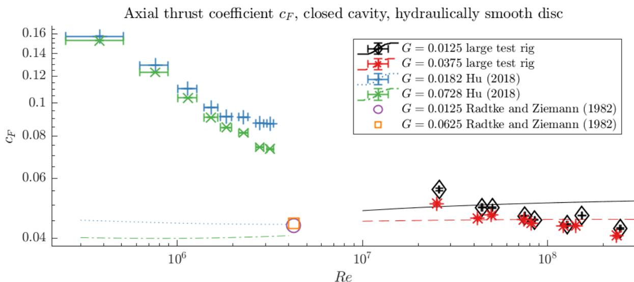
**Figure 4: Axial thrust coefficient of small and large test rig as well as from Radtke, Ziemann (1982). Markers are measurements; lines show the corresponding prediction from the models by Kurokawa and Sakuma (1988). Small test rig data is taken from Hu (2018).**
