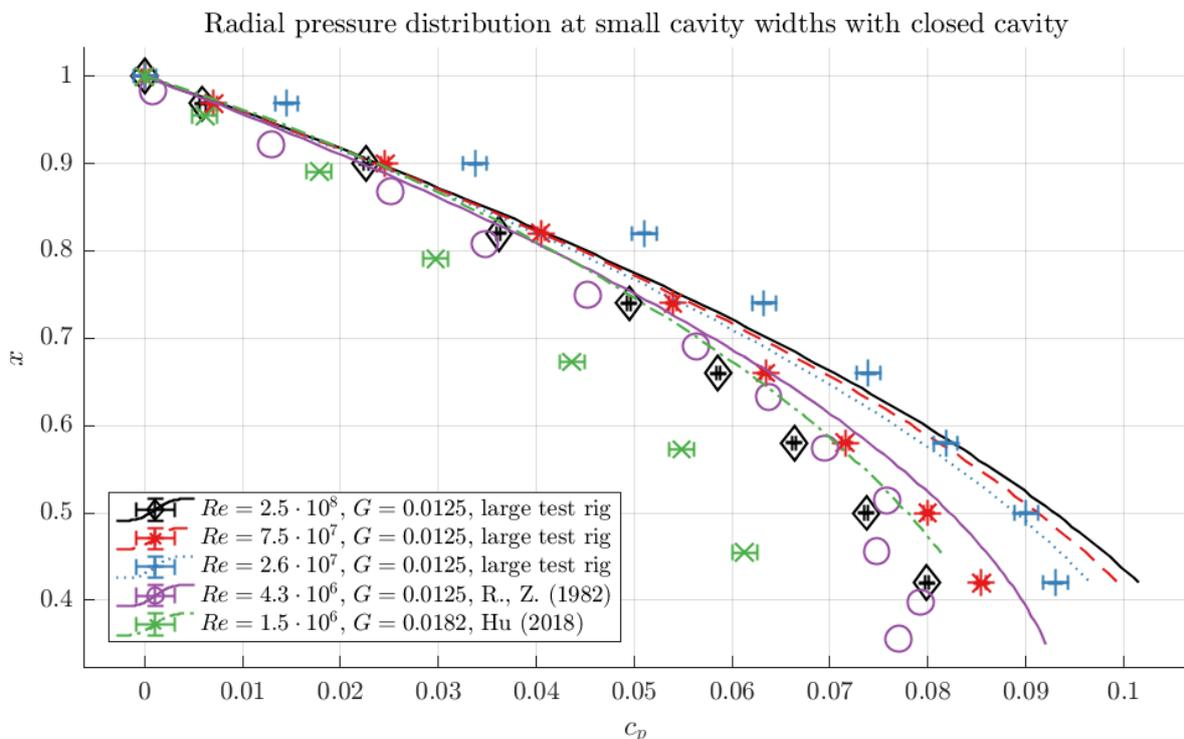
**Figure 3: Radial pressure distribution at small cavity widths with closed cavity. Markers denote measurements; lines are predictions from the models proposed by Kurokawa and Sakuma (1988).**
