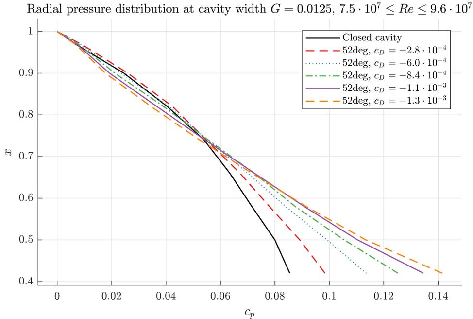
**Figure 9: Radial pressure distribution at relative cavity width  $G = 0.0125$ , Reynolds numbers  $7.5 \cdot 10^7 \leq Re \leq 9.6 \cdot 10^7$ , closed cavity and  $52^\circ$  preswirl angle with centripetal through-flow.**
