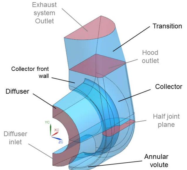
**Figure 2: Exhaust system sections and components**
