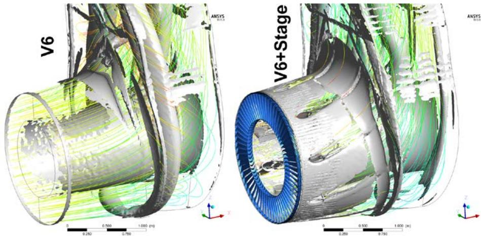
**Figure 9: Comparison between isolated and joint diffuser simulation**
