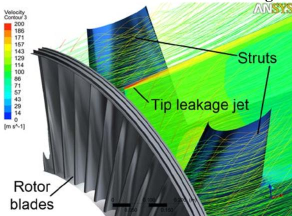
**Figure 7: Velocity streamline at tip region**
