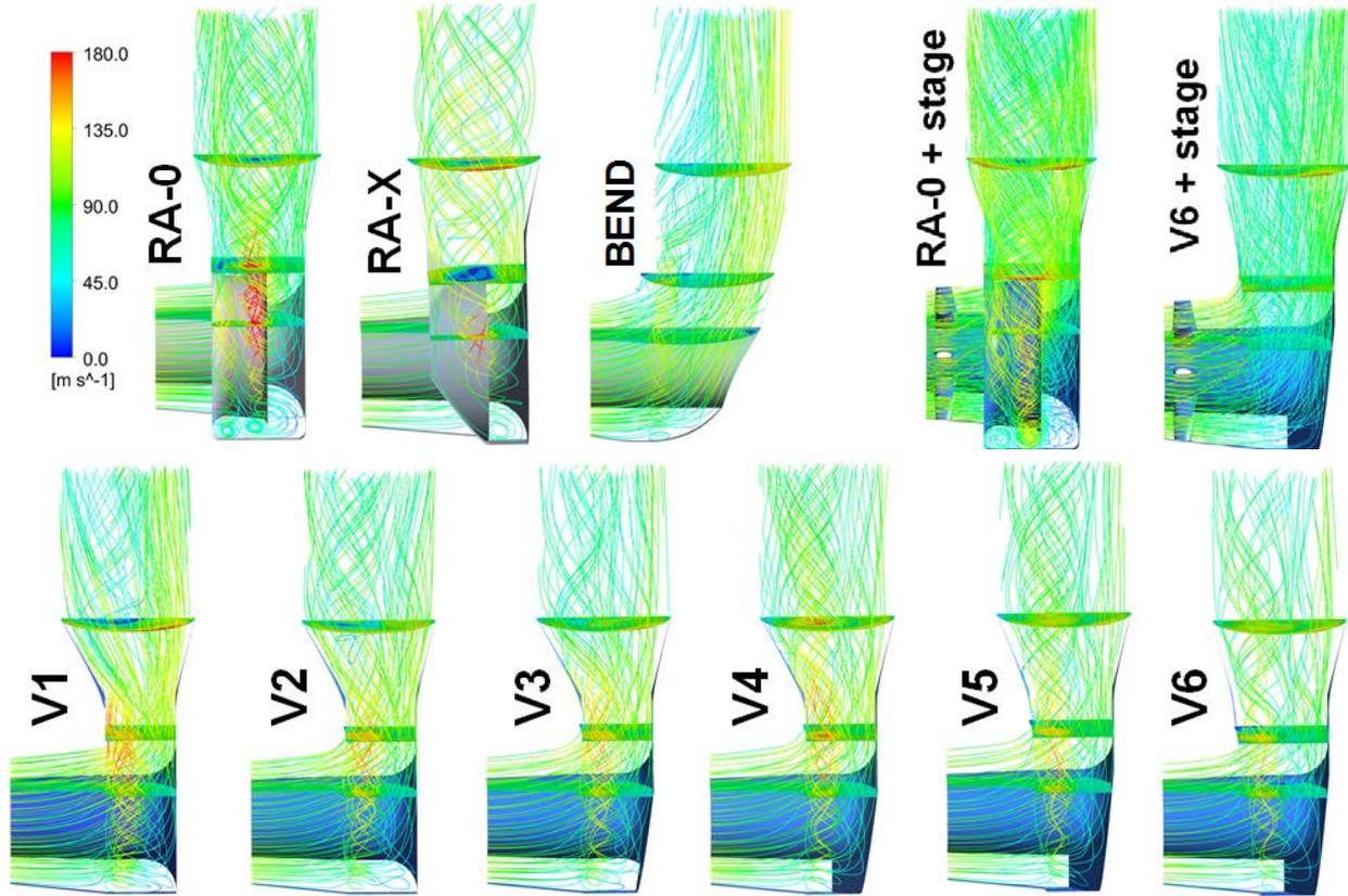
**Figure 6: Velocity streamlines**
