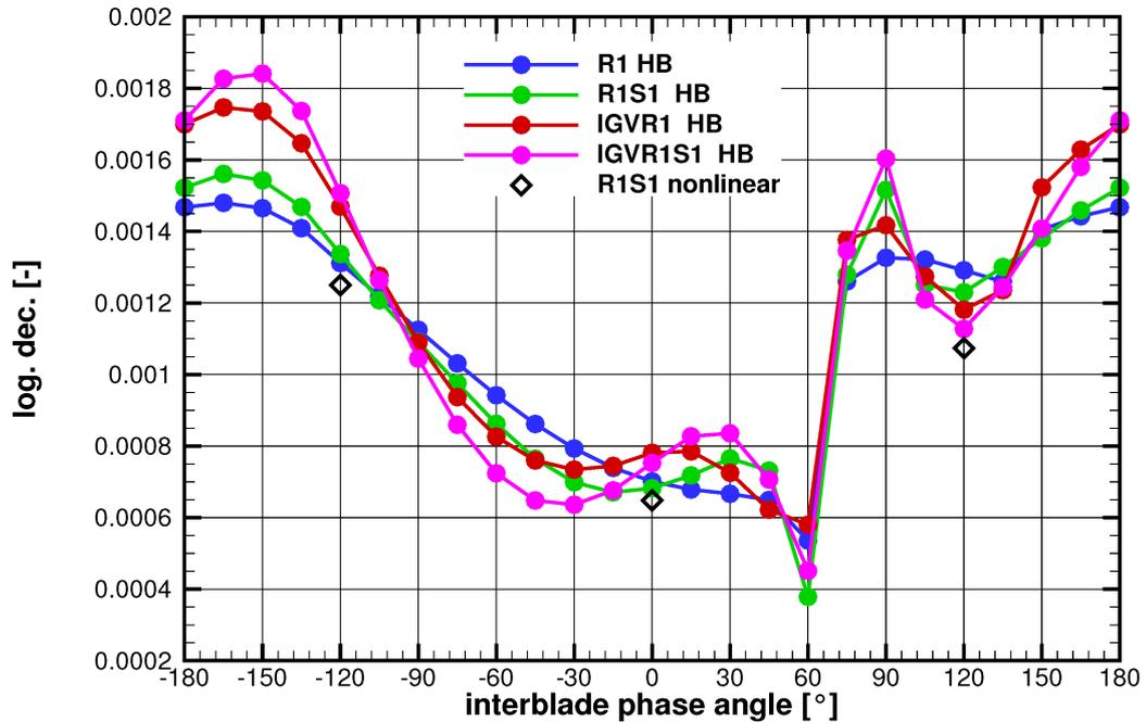
Figure 4: Aerodynamic damping (logarithmic decrement) for the embedded rotor.
