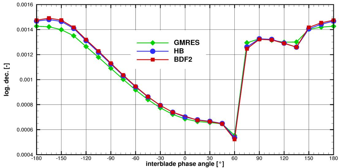
Figure 3: Aerodynamic damping (logarithmic decrement) for isolated rotor.
