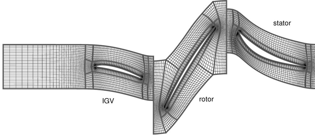
Figure 2: Mesh and block topology.
