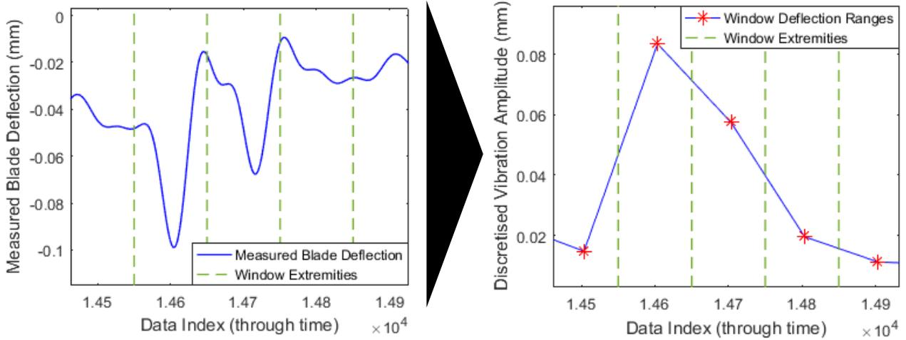
1. Measured vibration signal is discretised and local peak values identified.
