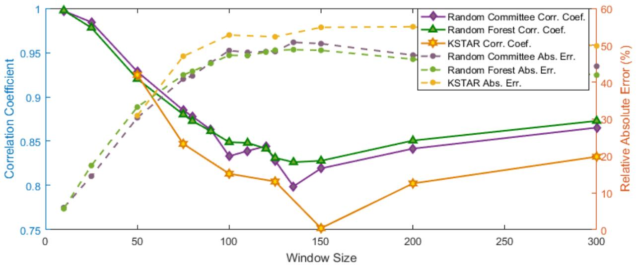
**Figure 7: Effect of discretisation window size, on vibration prediction accuracy of the three computational intelligence methods, for the “Envelope” discretisation method.**
