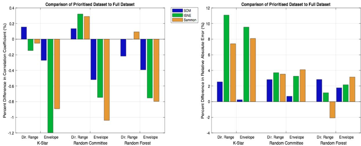
**Figure 10: Comparison of model performance of reduced datasets represented as a percent difference from the full dataset for different CI algorithms and discretisation methods. Correlation Coefficient (left); Relative Absolute Error (right)**
