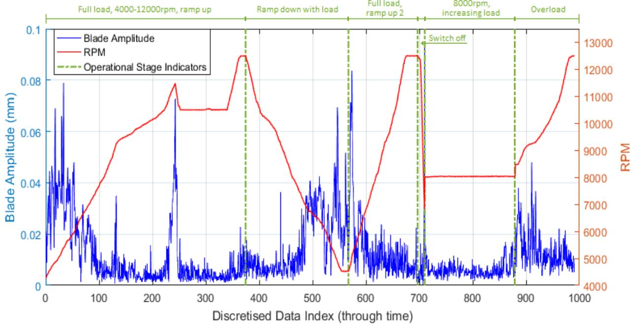
**Figure 1: Superposition of machine RPM and measured blade amplitude through time (blade #2, probe averaged, envelope discretisation, window size 50).**
