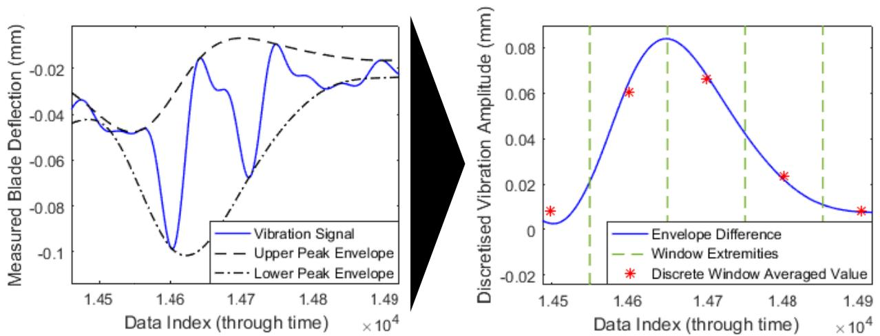
1. Spline envelope functions calculated above and below vibration signal.
