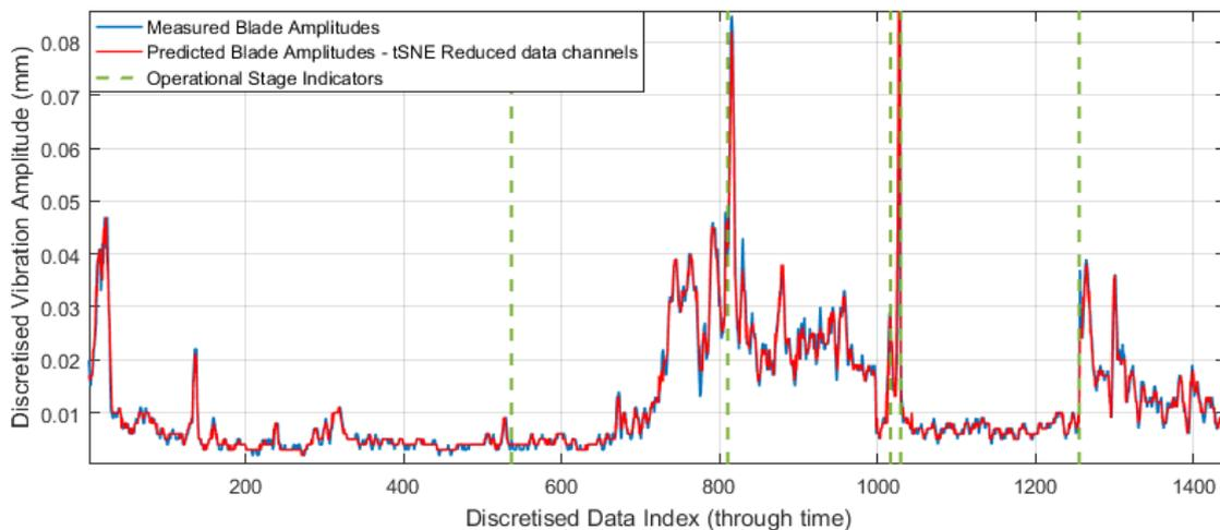
**Figure 11: Comparison of “best case” model with measured blade amplitudes.**
