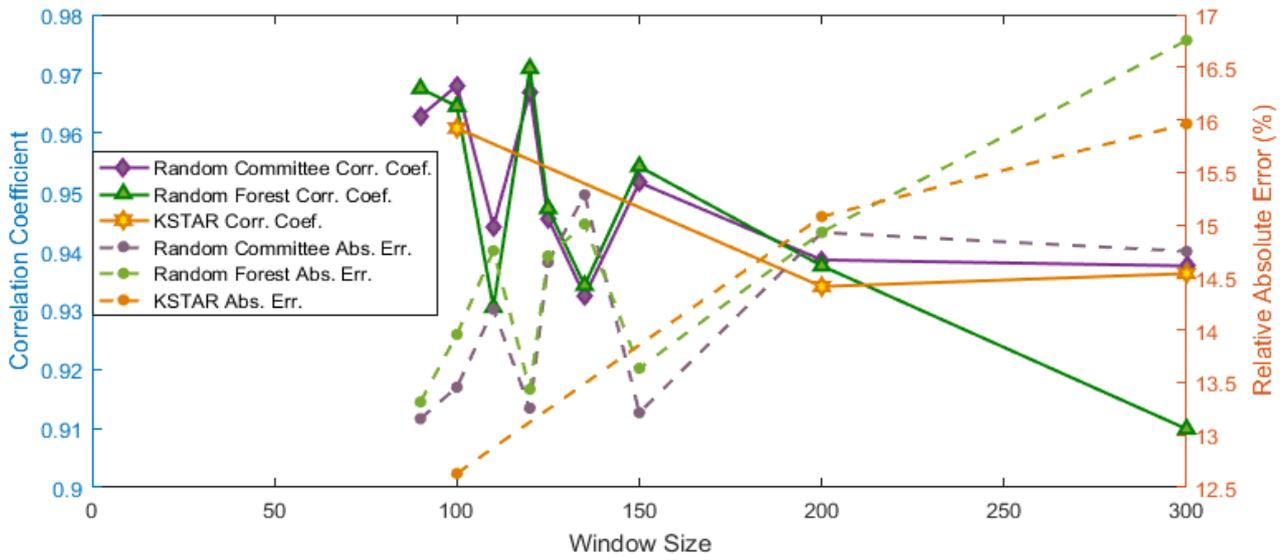
**Figure 6: Effect of discretisation window size, on vibration prediction accuracy of the three computational intelligence methods, for the “Direct-Range” discretisation method.**
