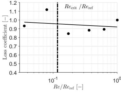
Figure 9: **Trailing edge loss coefficient. Altitude effect.**
