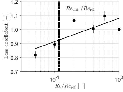
Figure 8: **Boundary layer loss coefficient. Scaling effect.**
