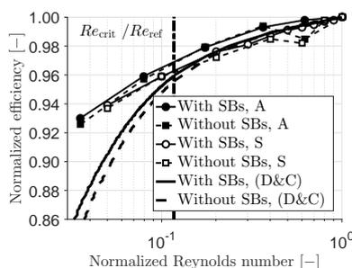
Figure 11: Change in specific entropy with a decreasing Reynolds number. Figure 12: Change in efficiency with a decreasing Reynolds number.
