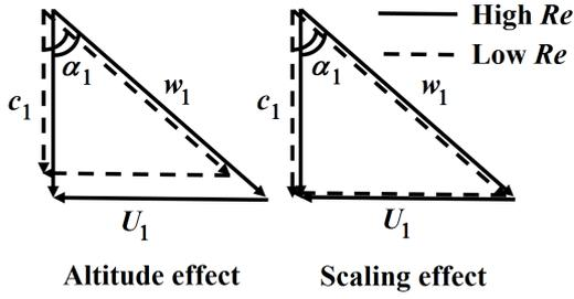
Figure 5: Velocity triangles at the impeller inlet.
