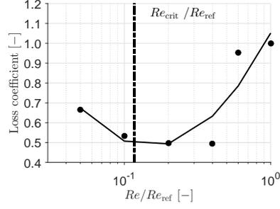
Figure 10: **Trailing edge loss coefficient. Scaling effect.**
