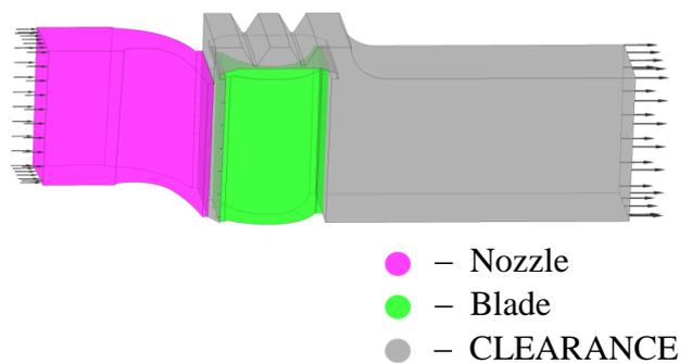
**Figure 8: 3D model of the turbine stage**
