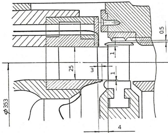
Figure 1: **The studied turbine stage drawing (all dimensions are in mm)**
