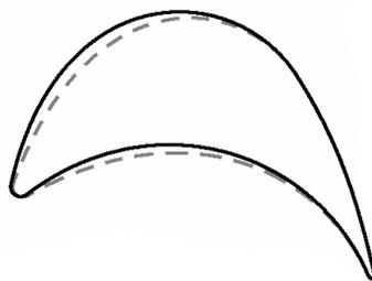
Figure 5: **Mean cut of the initial (—) and obtained (---) blade profile with incidence angle  $+3^\circ$**
