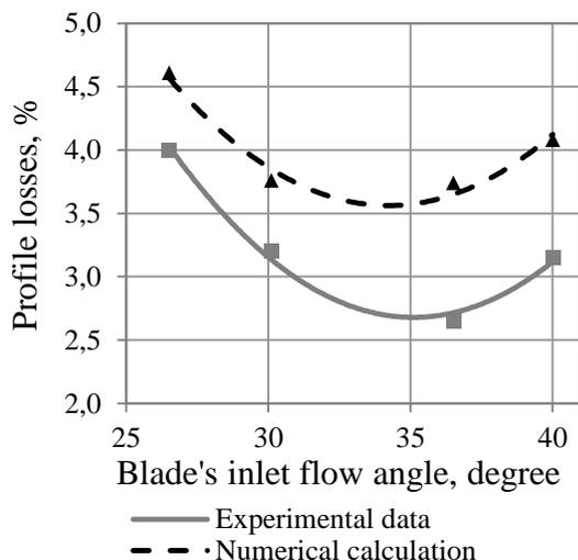
Figure 2: **Profile losses for the experimental data and the numerical calculations**
