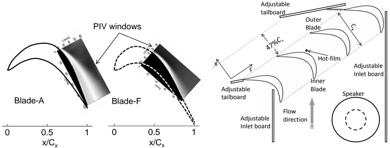
**Figure 1. Sketch of blade profiles (left) with PIV window location; schematic of the wind tunnel (right)**
