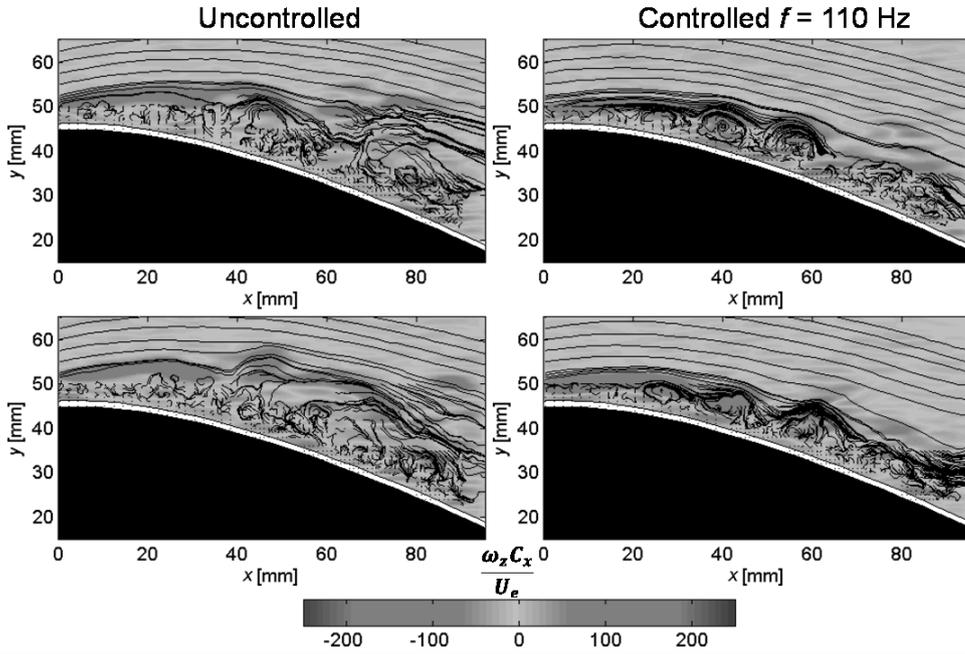
**Figure 4. Instantaneous PIV images at two instants for Blade-F, Low- $Tu$ : streamlines superposed on normalized spanwise vorticity contours ( $\omega_z C_x / U_e$ ). Left column: uncontrolled; right column: control at  $f = 110$  Hz.**
