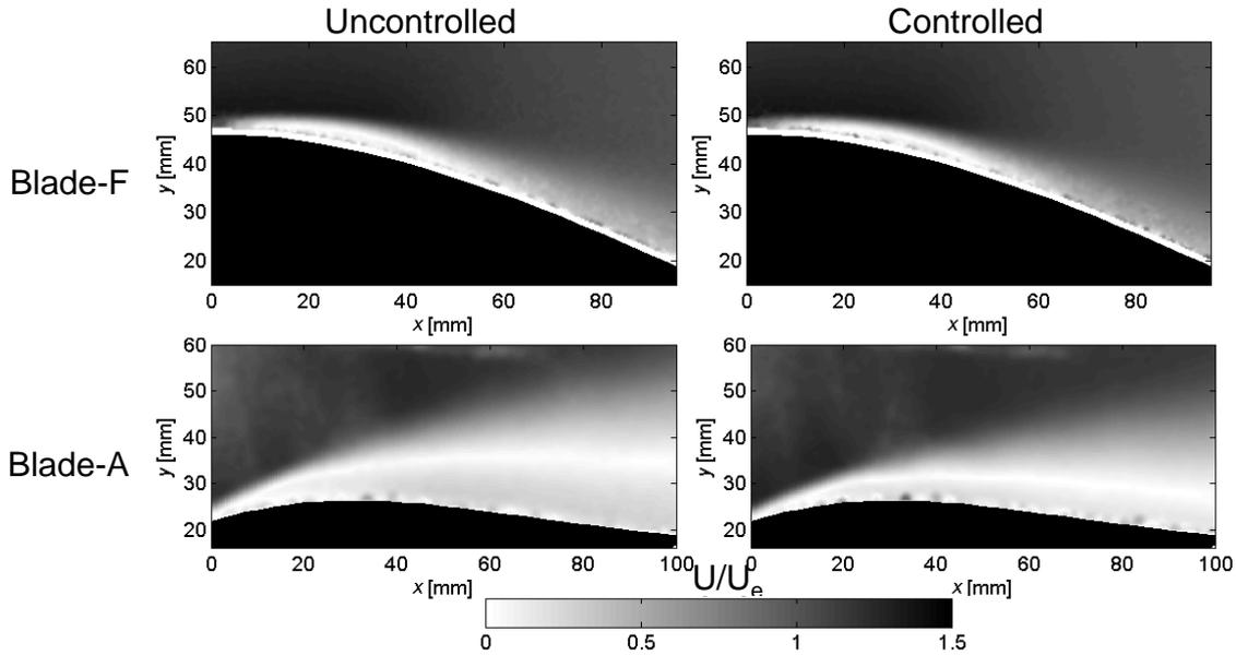
**Figure 5. PIV time-averaged velocity magnitude for Blade-F (top) and Blade-A (bottom), uncontrolled (left) and controlled (right) at  $f = 110$  Hz (Blade-F) and  $f = 130$  Hz (Blade-A).**
