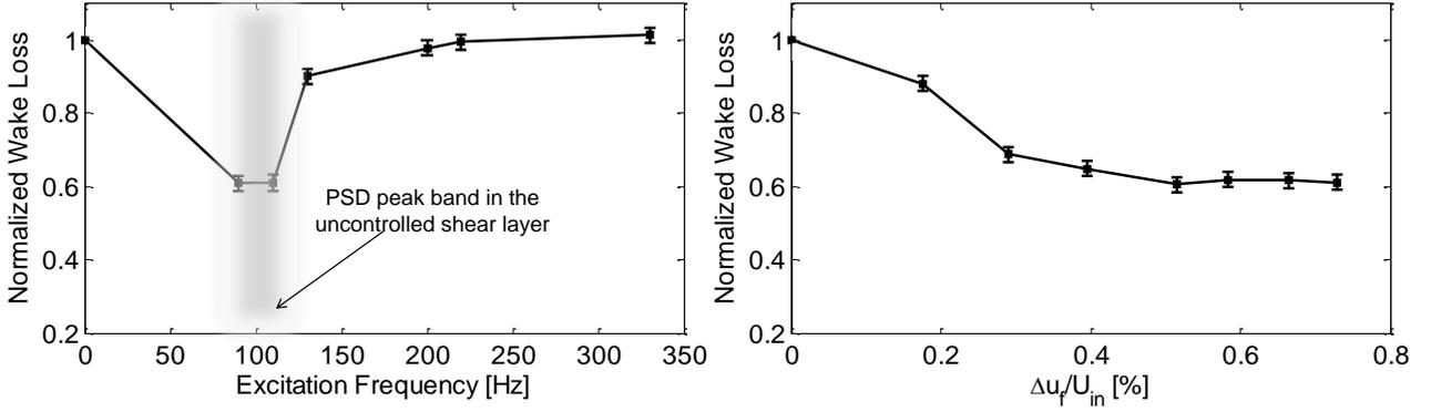
**Figure 3. Integrated wake loss coefficient normalized by the uncontrolled case for Blade-F, Low- $Tu$ . Left: excitation frequency effect. Right: amplitude effect, control at  $f = 110$  Hz.**
