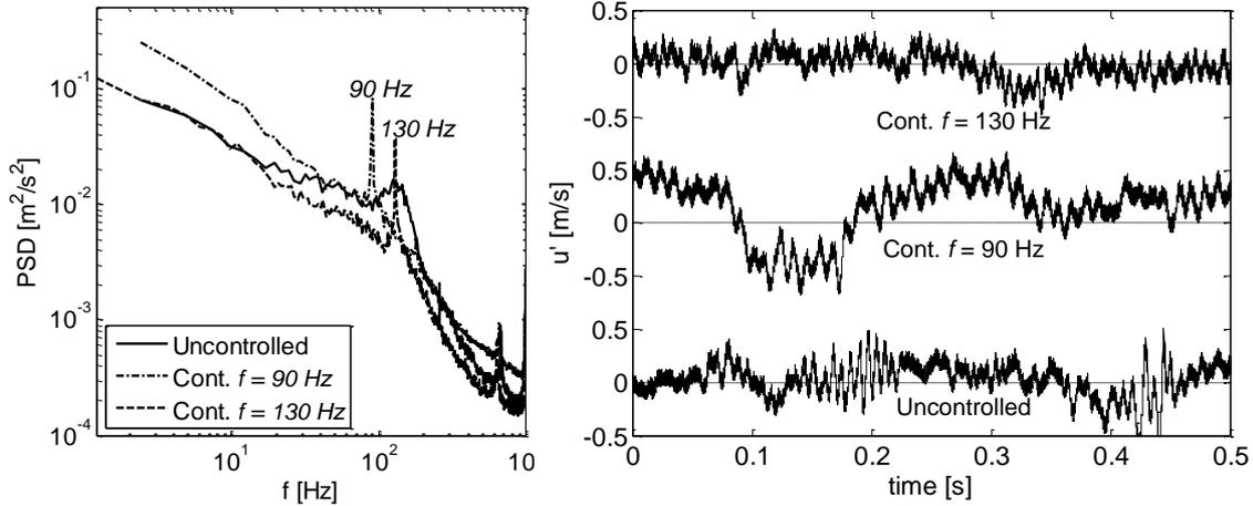
**Figure 7. Left: PSD of velocity signal at 70%  $C_x$  at negative peak skewness, Right: raw velocity fluctuations signal. Blade-A, high- $Tu$ , uncontrolled case and controlled cases at  $f = 90$  Hz and  $f = 130$  Hz.**
