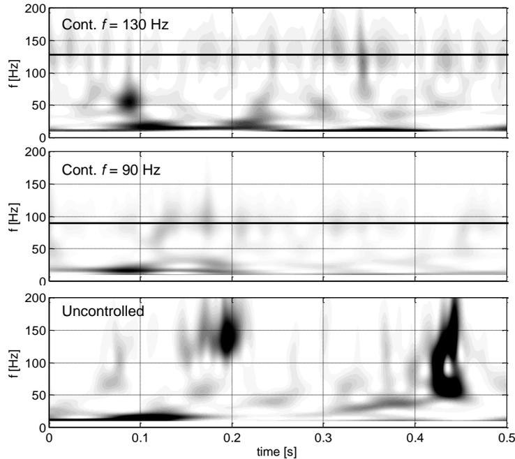
**Figure 8. Wavelet power contour of velocity signal at 70%  $C_x$  at negative peak skewness. Blade-A, high- $Tu$ , uncontrolled case and controlled cases at  $f = 90$  Hz and  $f = 130$  Hz.**
