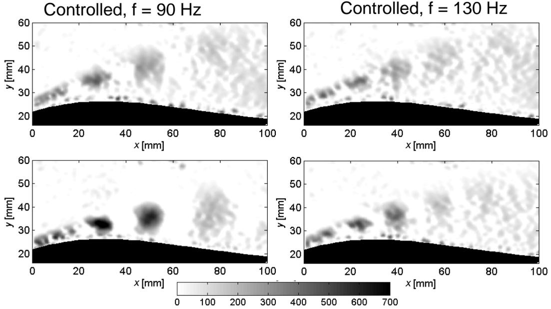
**Figure 9. Contours of swirl strength parameter from phase-locked PIV, Blade-A, high- $Tu$ , Control at:  $f = 90$  Hz,  $\Delta u_f/U_{in} = 0.5\%$  (top left),  $f = 90$  Hz,  $\Delta u_f/U_{in} = 1.8\%$  (bottom left),  $f = 130$  Hz,  $\Delta u_f/U_{in} = 0.5\%$  (top right),  $f = 130$  Hz,  $\Delta u_f/U_{in} = 1.1\%$  (bottom right).**
