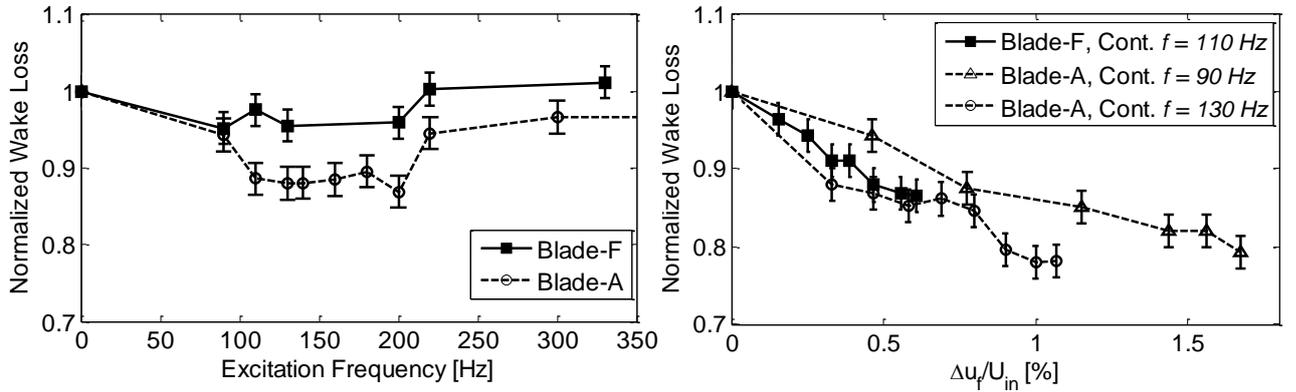
**Figure 6. Integrated wake loss coefficient normalized by the uncontrolled case for Blade-F and Blade-A, High- $Tu$ . Left: excitation frequency effect. Right: amplitude effect.**
