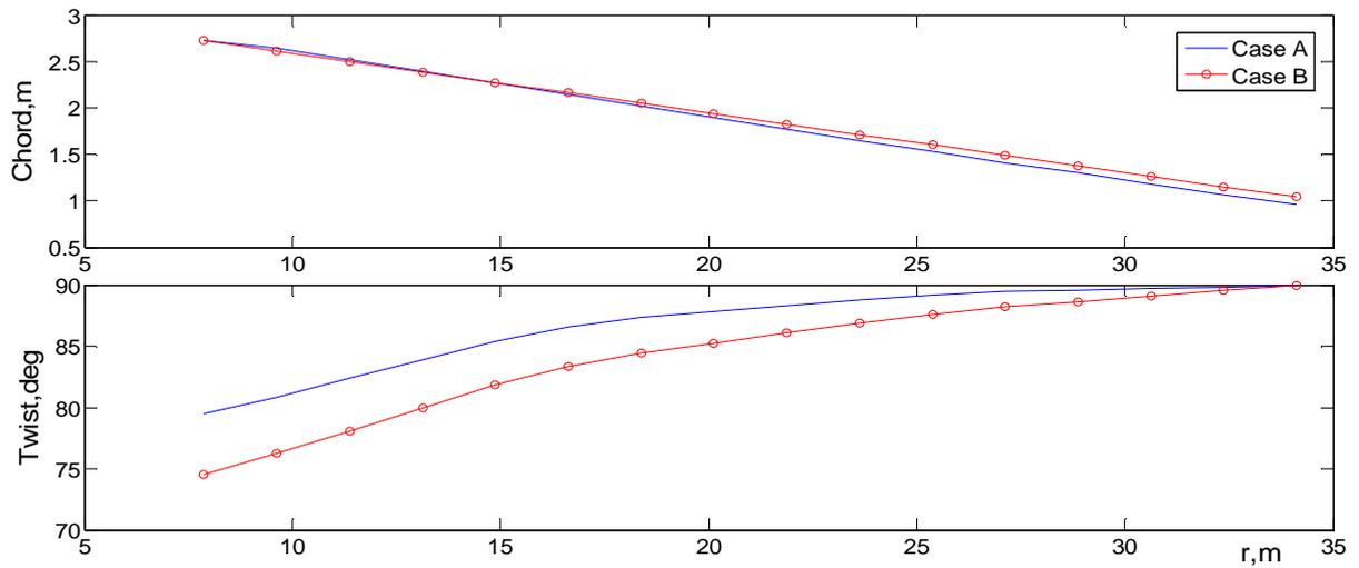
Figure 8. Chord and twist distributions for cases A and B
