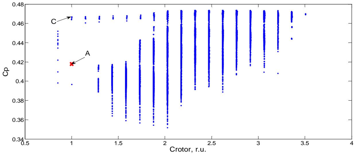
Figure 9. Power coefficient versus rotor cost for different chord, twist and cross-sectional distributions
