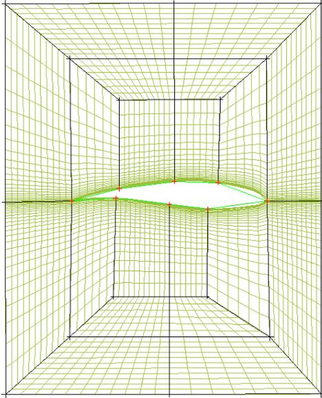
**Figure 13. O-grid around the blade section (axi-radial plane).**
