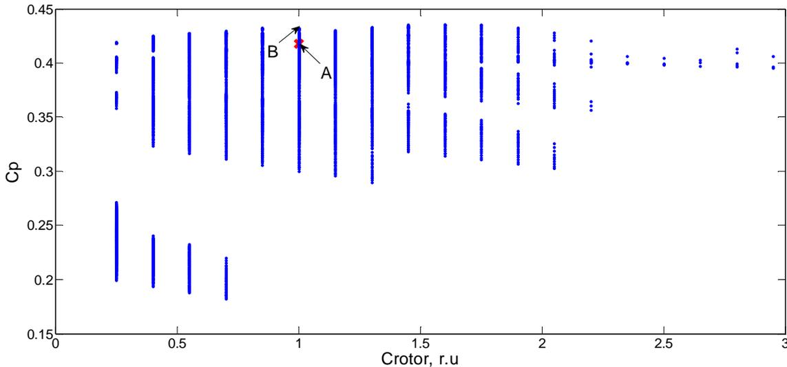
**Figure 7. Power coefficient versus rotor cost for different chord and twist distributions**
