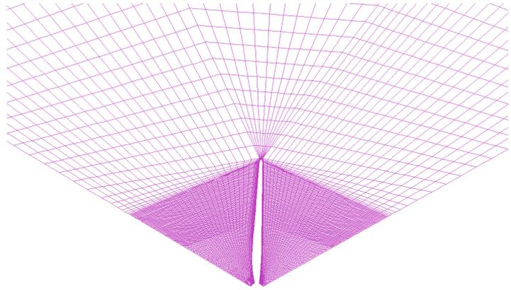
**Figure 14. Mesh around the blade section (meridional plane).**
