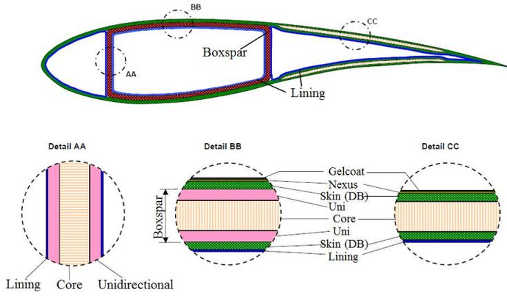
**Figure 3. Structural layout of composite blade. Based on Bir and Migliore (2004)**
