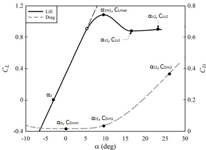
**Figure 2. Lift and drag curves coding, based on Merz (2011)**
