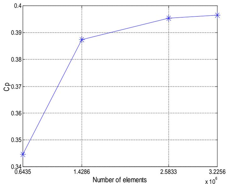
**Figure 15. Dependence of power coefficient on the grid size.**
