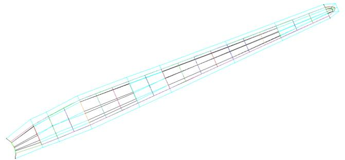
Figure 12. 3D block topology model around the blade
